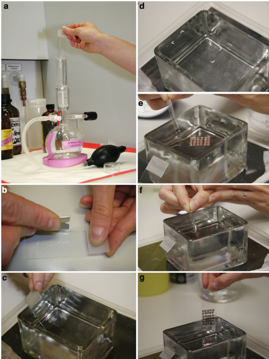
Fig. 4. Steps required for coating of grids. (a) Clean glass slide dipped inside the coating device containing the formvar solution. (b) Slide coated with formvar, cut by a razor blade to separate the film. (c) Slide with cut film dipped inside the water-containing cuvette to separate the film from the glass slide. (d) Grey film floating on top of the clean water (corners marked by white angles ). (e) Grids are arranged on top of the thin film and the free end is used to pick up the grid along with the film. (f) Grids with the film are now sticking to the coverslip inside water. (g) Lifting of the grids from the water.
