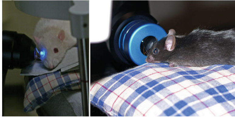
Fig. 5. Examples for rat and mouse positioning in front of the SPECTRALIS® device. Due to the flexibility of the used cherry stone filled pad, rodents of different sizes can be placed stable in various positions.
