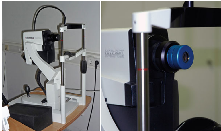
Fig. 2. The SPECTRALIS® HRA + OCT device by Heidelberg Engineering. On the right, the device is shown with the attached additional lens to facilitate imaging of small rodent's eyes.
