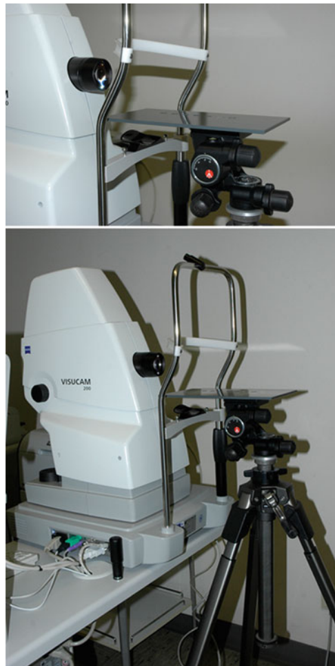
Fig. 3. Zeiss Visucam® 200 with an altered tripod for mouse positioning.
