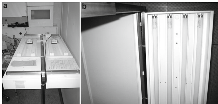
Fig. 1. Light exposure device. (a) View from top. (b) View from below showing the mounting of the light bulbs. The bulbs on the left side are shielded by the diffusion screen. On the right side of the device, the screen has been removed to reveal the arrangement of the light bulbs.
